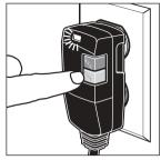
**Step 2**If the GFCI light glows, press the "Test" button until the light goes out.
